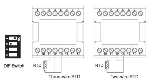
Figure 2.6 RTD Input Wiring
