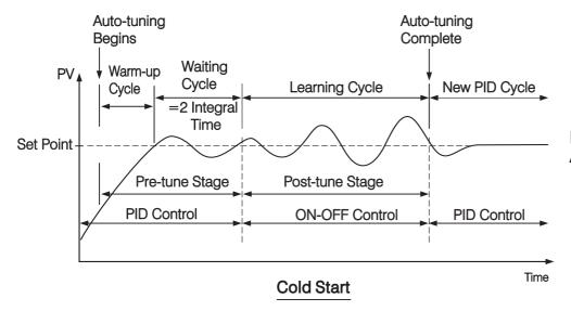
Figure 3.22 Auto-tuning Procedure
