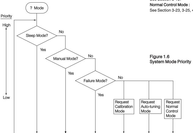
The calibration mode, auto-tuning mode and normal control mode are in the same priority level. The sleep mode is in the highest priority.
