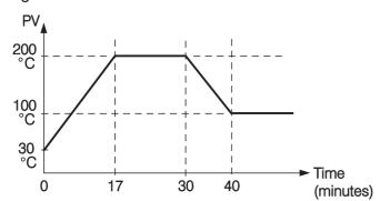
Note: When the ramp function is used, the lower display will show the current ramping value. However it will revert to show the set point value as soon as the up or down key is touched for adjustment. The ramping value is initiated to process value either power up or RAMP and /or set point are changed. Setting RAMP to zero means no ramp function at all.
