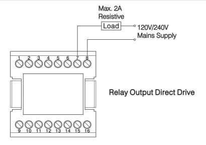
Figure 2.16 Alarm 1 Wiring
