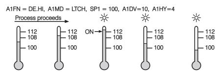
Figure 3.10 Latching Deviation Alarm
