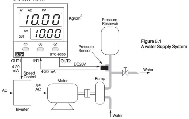
The water pressure is required to be controlled at 10 Kg/cm<sup>2</sup>, to achieve this, the following devices are used for this example:
