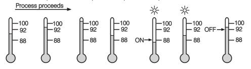
Figure 3.11 Holding Deviation Alarm
