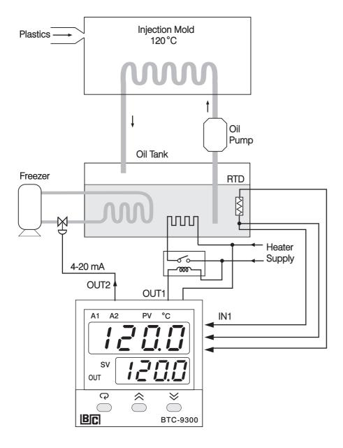
Figure 5.7 Heat-Cool Control Example
