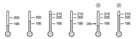
Figure 3.8 Latching / Holding Process Alarm
