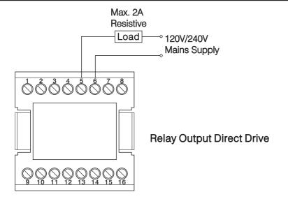
Figure 2.14 Output 1 Wiring
