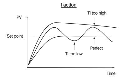
Figure 3.25 (Continued ) Effects of PID Adjustment
