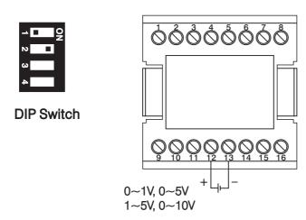
Figure 2.7 Input 1 Linear Voltage Wiring
