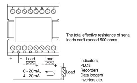
Figure 2.22 Analog Retransmission Wiring
