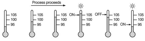
Figure 3.15 Holding Deviation Band Alarm
