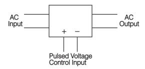
Figure 5.2 Block Diagram of VPFW SSR
