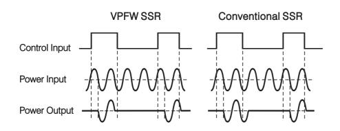
Figure 5.3 VPFW SSR vs. Conventional SSR
