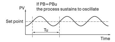
Figure 3.24 Critical Steady State
