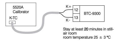
The 5520A calibrator is configured as K type thermocouple output with internal compensation. Send a 0.00 °C signal to the unit under calibration.
