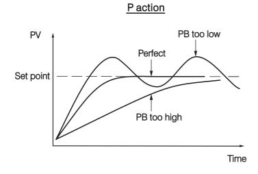
Figure 3.25 Effects of PID Adjustment
