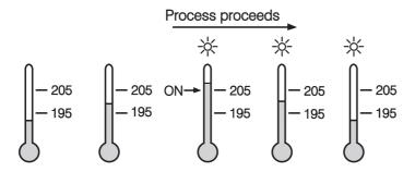
Figure 3.6 Latching Process Alarm
