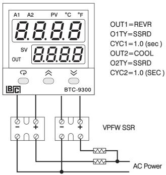
Figure 5.4 VPFW SSR Application Example
