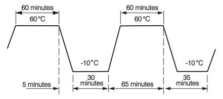
Figure 5.9 Temperature Profile of Chamber
