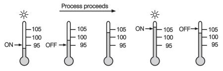
Figure 3.13 Normal Deviation Band Alarm
