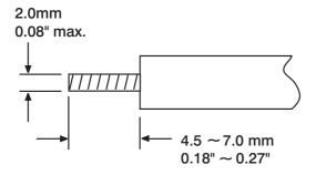
Figure 2.2 Lead Termination
