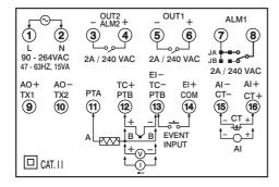
Figure 2.3 Rear Terminal Connection Diagram
