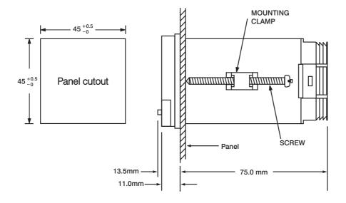
Figure 2.1 Mounting Dimensions
