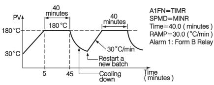
Figure 5.11 Temperature Profile of Baking Oven
