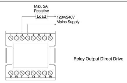
Figure 2.15 Output 2 Wiring
