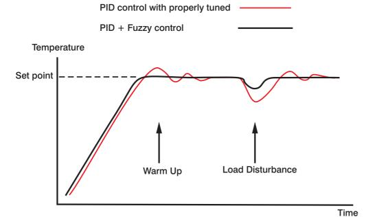
Figure 1.2 Fuzzy PID Enhances Control Stability
