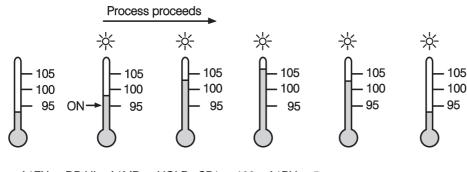
Figure 3.14 Latching Deviation Band Alarm
