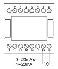
Figure 2.10 Input 2 Linear Current Wiring
