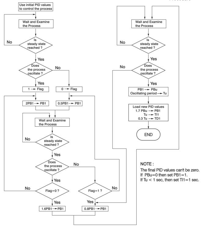
The above procedure may take a long time before reaching a new steady state since the P band was changed. This is particularly true for a slow process. So the above manual tuning procedures will take from minutes to hours to obtain optimal PID values.
