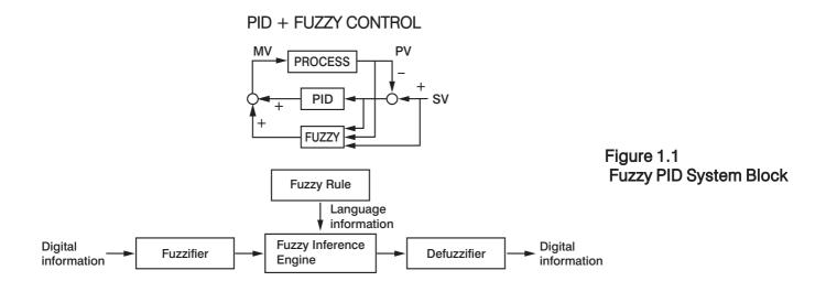
The function of Fuzzy Logic is to adjust PID parameters internally in order to make manipulation output value MV more flexible and adaptive to various processes. The Fuzzy Rule may work like these:
