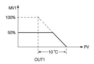
Figure 4.5 Power Limit Function
