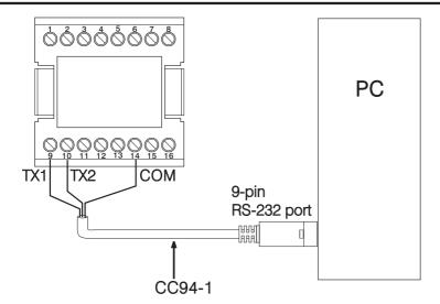
Figure 2.19 RS-232 Wiring
