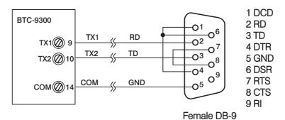
Figure 2.21 Configuration of RS-232 Cable
