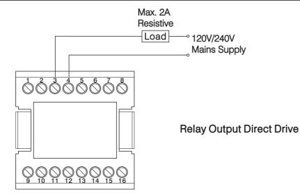
Figure 2.17 Alarm 2 Wiring
