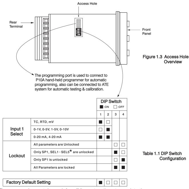
The programming port is used for off-line automatic setup and testing procedures only. Don't attempt to make any connection to these pins when the unit is used for a normal control purpose.
