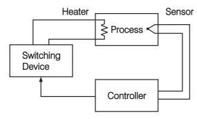
Figure 3.18 Loop Break Sources
