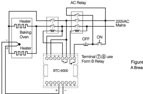
Figure 5.10 A Bread Baking Oven
