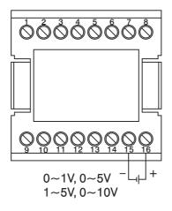
Figure 2.9 Input 2 Linear Voltage Wiring
