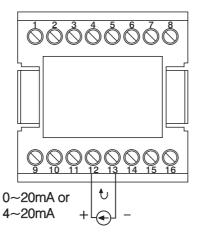
Figure 2.8 Input 1 Linear Current Wiring
