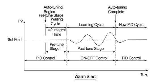
If the auto-tuning begins near the set point (warm start), the unit passes the warm-up cycle and enters the waiting cycle. Afterward the procedures are same as that described for cold start.
