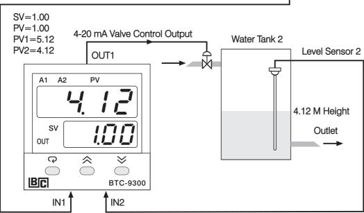
Adjust SP1( here is 1.00) to control the difference between PV1 and PV2. Choosing P1-2 for PVMD, the PV display will show the difference value ( PV1-PV2) between PV1 and PV2, and this value will be stabilized to the set point ( here is 1.00).
