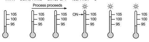
Figure 3.16 Latching /Holding Deviation Band Alarm
