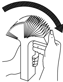
Fig. 5.5 Loosening the Chart Paper
