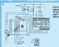
In A maintains the level between the on and off probes and activates the alarm when the liquid falls below the "low alarm" probe.
