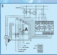
In A maintains the level between the on and off probes and activates the alarm in the liquid exceeds the "high alarm" probe.
