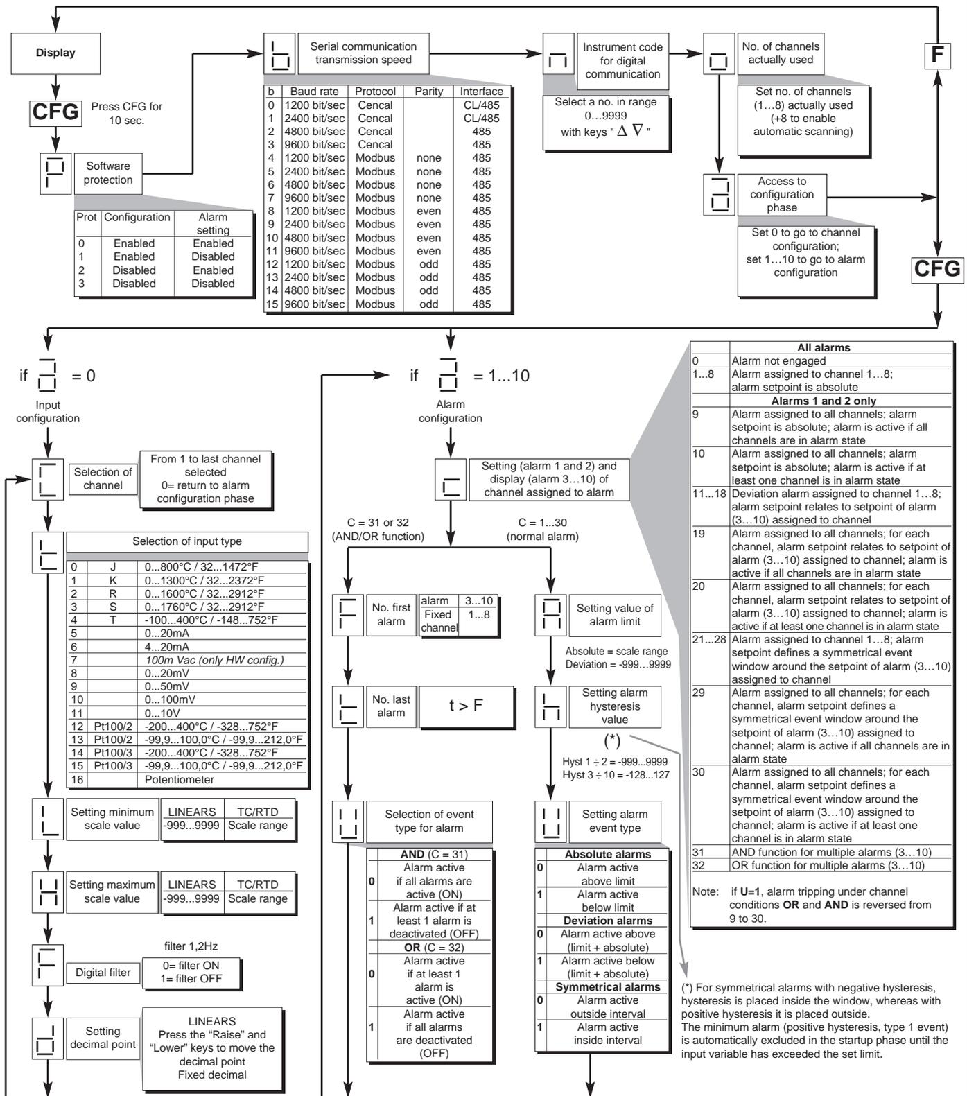
Move from one configuration phase to another by pressing the CFG key; press the F key to go to display.
