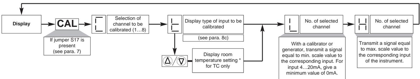
**ATTENTION:** the instrument is supplied calibrated; any additional calibration must be made by a trained technician equipped with the necessary devices. The procedure is irreversible.
