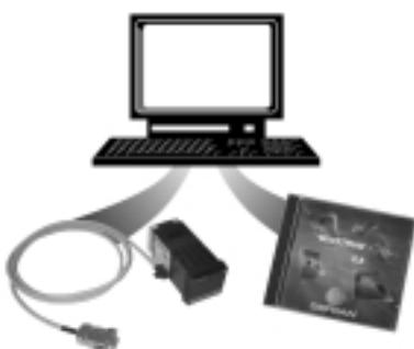
**N.B.** RS232 interface for PC configuration is supplied with the WINSTRUM programming software. Make connection with instrument powered but with inputs and outputs disconnected.
