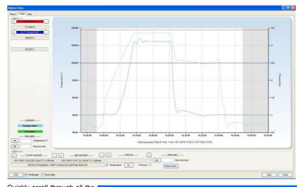
Set vertical and horizontal markers for your analysis and statistics, zoom in the graph in the most important phases of the current process, customize the grid according to your needs. You have plenty of options in the graph tab and all are user-friendly and quick to set. The Seal function is used to close an analysis and avoid possible further modifications to it.
