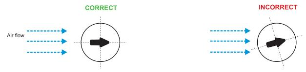
The mounting flange allows for precise setting of the EE660 immersion depth in a duct. The entire sensing head must be in the air flow to be measured.
