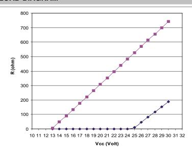
The diagram shows the optimum ratio between load and power supply for transmitters with 4...20mA output.
