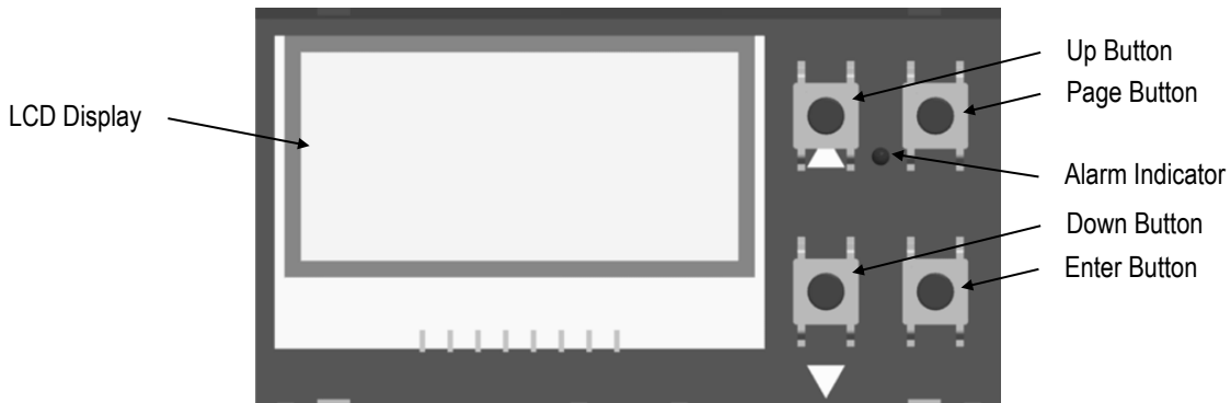
Figure 33: Control Panel for the Comm Box (DIN)
