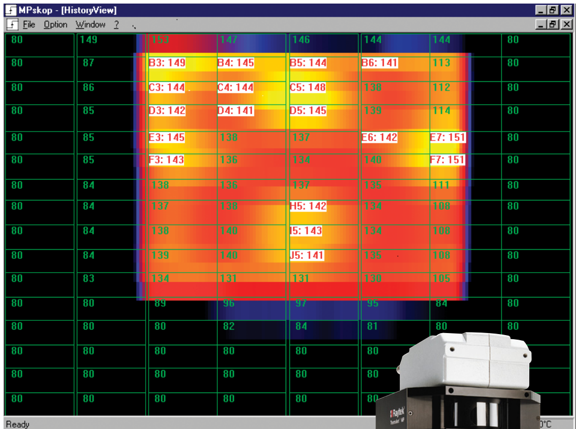
Thermal image from actual thermoforming application
