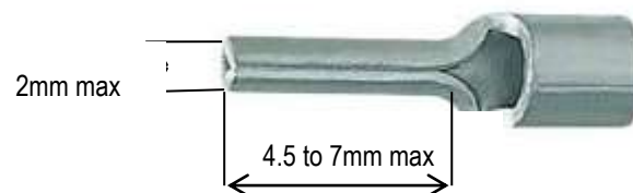
2-15. Lead Terminal for C22
