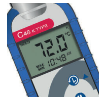
Max/Min feature recalls highest and lowest reading
